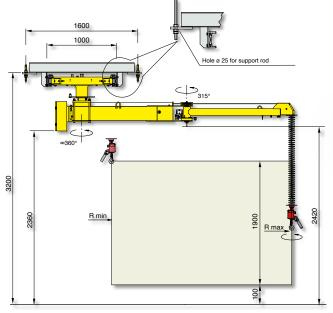
Air supply: dry and oil-free compressed air min. constant 0.7÷0.8 MPa
