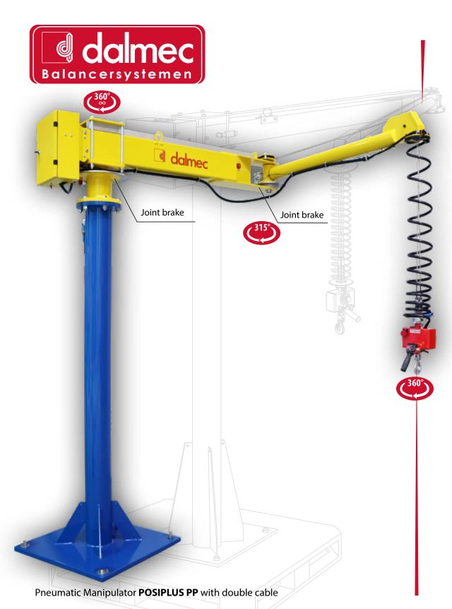
POSIPLUS PP, is a double cable manipulator with high load capacities, it is able to handle loads up to 200 kg and reaches working radii up to 4500 mm. The gripping tool is connected to the balancing group through two independent steel cables to ensure maximum safety. The particular double-arm structure with intermediate joint makes it easy to operate within the entire working area. Specific brakes mounted on the main joints guarantee control of drift movements.
